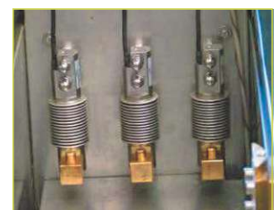
Detail: 3 load cells 500 N
