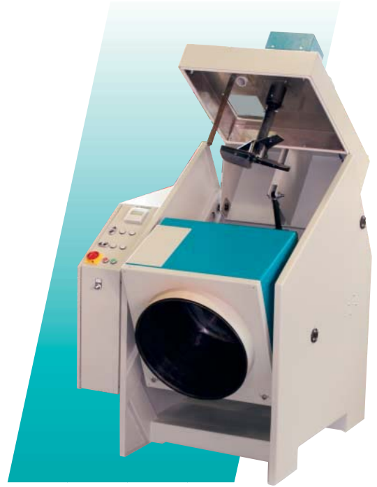
Mischtrommel in Entleerstellung Mixing drum tilted for emptying
