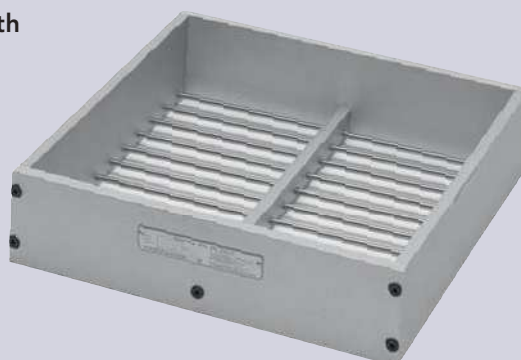
Grid Sieve according to EN 933-3
